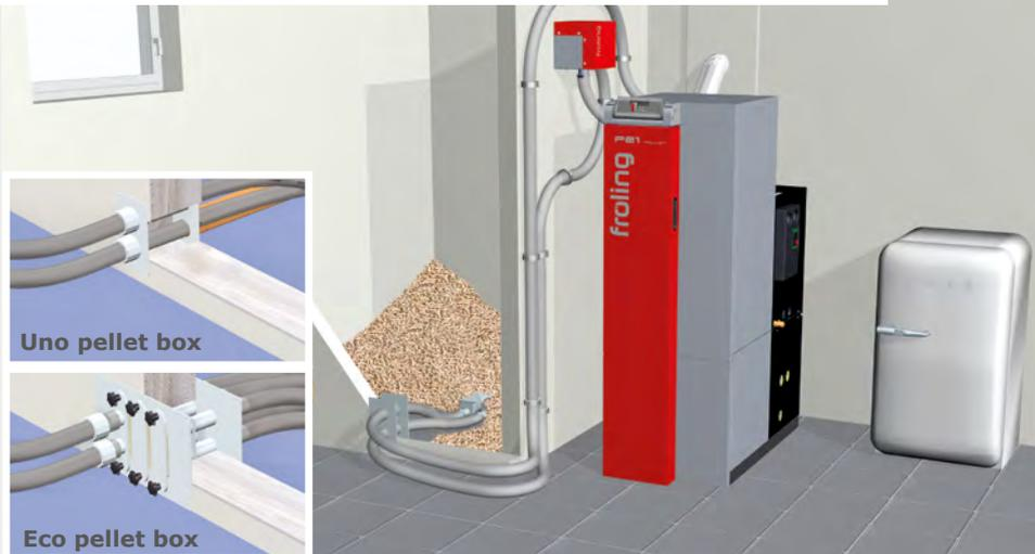
The suction system can handle even large distances between the store and the boiler room. The position of the suction probes and the transfer unit can be adjusted to suit the individual store conditions. The changeover between suction probes is manual (**Eco pellet box**). There is also a version of the suction system specially for square rooms with an individual probe (**Uno pellet box**).
