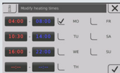
Fig. 2 View of the heating times (individually adjustable)
