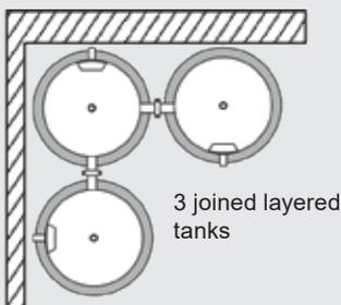
The layered tanks can either be set up in a row or at an angle: In this case the connection couplings are fitted to the layered tank in the middle at an angle of 90°.
