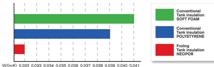
Neopor<sup>®</sup> is the latest version of the insulating material Styropor<sup>®</sup>. The foam polystyrene contains graphite particles which reduce the thermal radiation and therefore heat loss.
