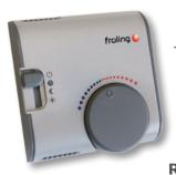
The main modes of the designated heating circuit can be easily adjusted and selected using Froling's **FRA room temperature sensor**. The adjusting wheel allows you to change the room temperature by up to  $+/-3^{\circ}$  C.
