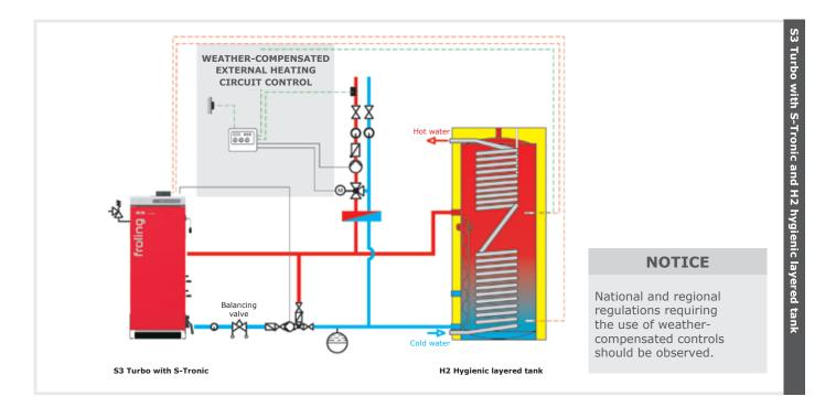
The **Lambdatronic controllers** allow for efficient energy management. Up to 4 storage tanks, up to 8 hot water tanks and up to 18 heating circuits can be integrated into the heating management system. You also benefit from the ability to integrate other means of energy production, such as solar panels.
