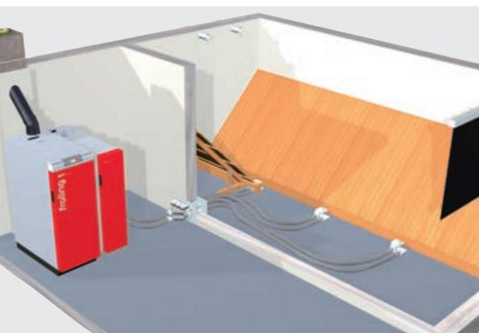
With its easy to install features, the universal suction system is equipped to handle large distances between the storage place and the boiler room. The position of the suction probes or the transfer unit (pellet box) can be adjusted to fit the conditions of the storage optimally.
