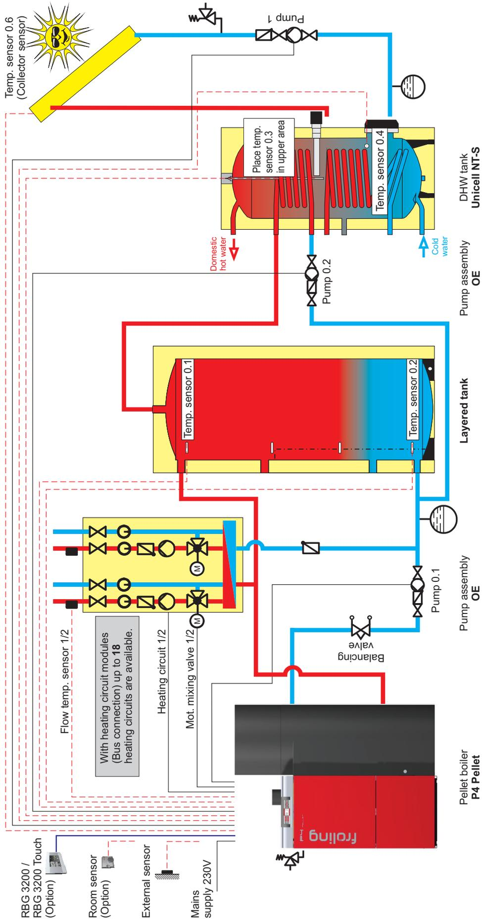
**Note:** When a storage tank is used, always set the parameter in menu BOILER, item SERVICE, VARIABLE MODE ACTIVATED to "NO"! Set parameter in menu SOLAR, item SERVICE, SOLAR SYSTEM to "1", WHICH SENSOR IS USED FOR THE SOLAR COLLECTOR to "0.6", WHICH PUMP IS USED FOR THE SOLAR COLLECTOR to "Pump 1". Controller P 3200, Since version 50.04 B04.08
