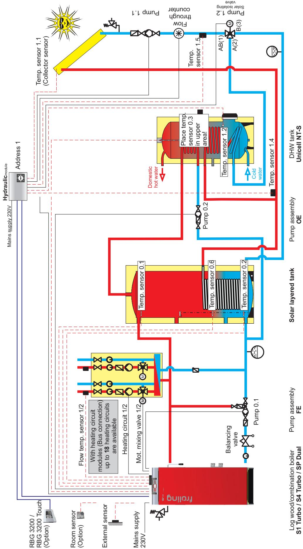
**Note:** Please set parameter in menu SOLAR, item SERVICE, SOLAR SYSTEM to "3", item SOLAR HEAT METER, WHICH SENSOR IS USED FOR HEAT METER FLOW TEMPERATURE to "1.4". Controller S3200
