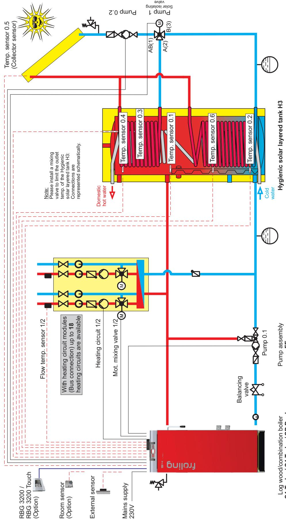
**Note:** Please set parameter in menu SOLAR, item SERVICE, SOLAR SYSTEM to "3", WHICH SENSOR IS USED FOR THE SOLAR COLLECTOR to "0.5", WHICH PUMP IS USED FOR THE SOLAR COLLECTOR to "0.2", WHICH PUMP IS USED FOR THE SOLAR ISOLATING VALVE to "Pump 1", WHICH SENSOR IS USED FOR THE STORAGE TANK REFERENCE to "0.6". Controller S3200
