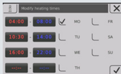
Fig. 2 View of the heating times (individually adjustable)
